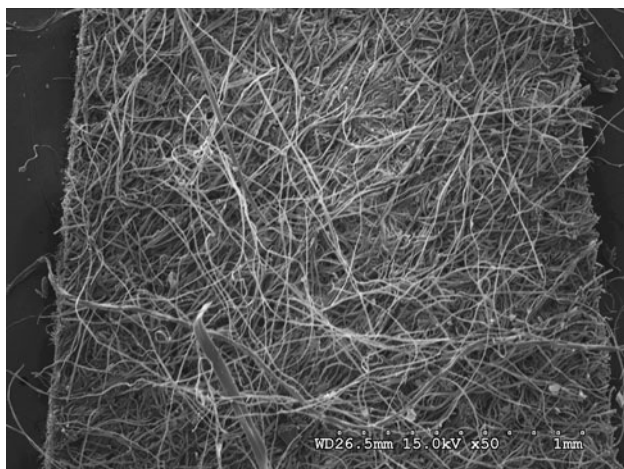
Fig. 3 SEM image of the surface of the bag worm cocoon shows the random orientation of the silk fibers that helps to create a firm cocoon
